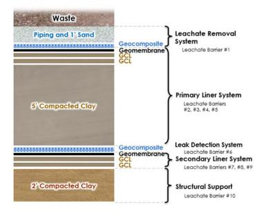
The liner system contains the disposed waste, collects and removes liquids entrained in the waste, and prevents the flow of liquid into the surrounding environment.
